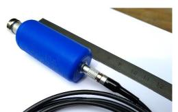
Lightweight sensor and magnet: < 10 g for high bandwidth
